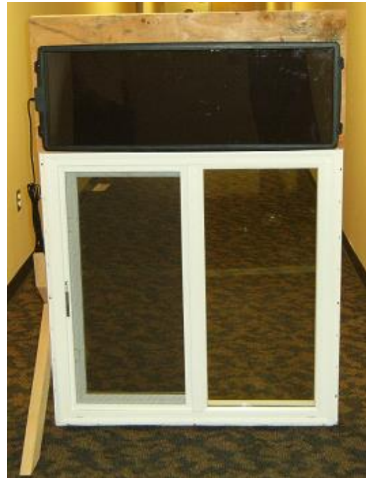
Fig. 12.14. Prototype of the Solar-Powered Automated Window.
